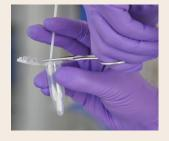
© Cut the swabs right above cotton part of the swab tip with a pair of scissors. Let the swab tip fall into a labeled tube (2ml or 5 ml) and close the lid. In case swabs are pooled it's possible to put multiple swabs into one tube.
