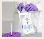
© Also put the tubes that contain the Feacal samples and swabs tips into the biohazard bag.
